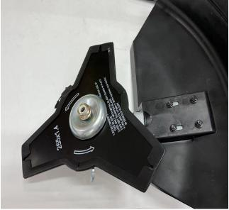
To remove the blade, insert a metal locking tool through the hole on the side of the drive sprocket and on the drive shaft. Loosen the clamp nut, then remove all parts.
