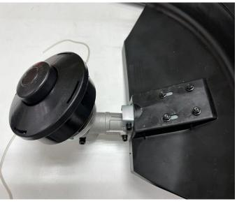
To disassemble the cutting head, insert a metal locking tool through the hole on the side of the drive sprocket and on the drive shaft. Unscrew the cutting head to remove it.
